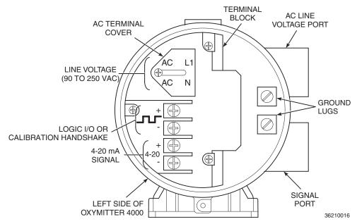
Figure A-2. Terminal Block and Wiring
